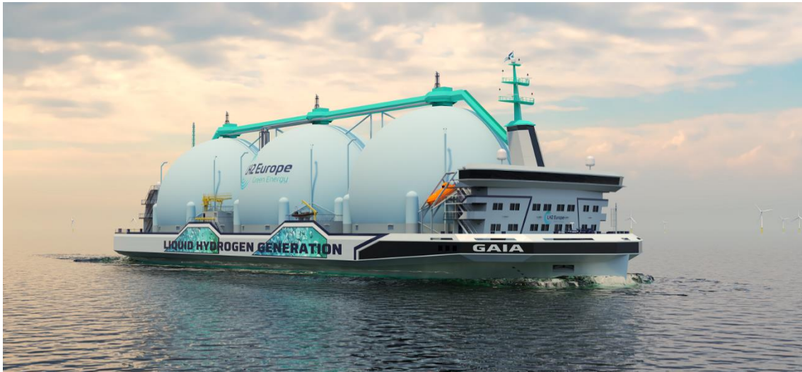
Abbildung 17: Design eines LH2-Wasserstofftankschiffs von LH2 Europe (LH2 Europe et al., 2022). Artist impression of the liquid hydrogen carrier design by LH2 Europe and C-Job Naval Architects.
